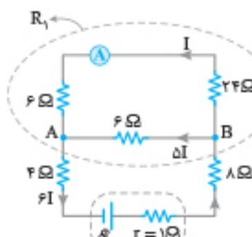
$$R_{eq} = \frac{I_1}{I_2} \Rightarrow \frac{I_1}{I_2} = \frac{30}{6} \Rightarrow I_1 = 5I$$
