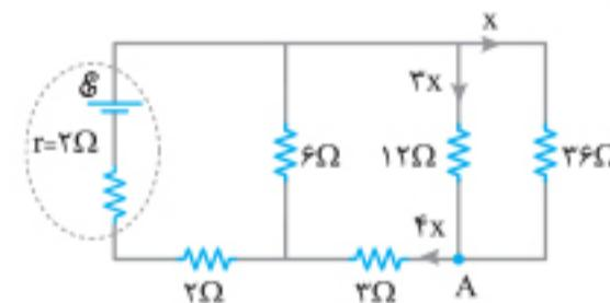
$$\frac{I_{36\Omega}}{I_{12\Omega}} = \frac{12}{36} \Rightarrow \frac{I_{12\Omega}}{I_{12\Omega}} = \frac{1}{3} \Rightarrow I_{12\Omega} = 3X$$
